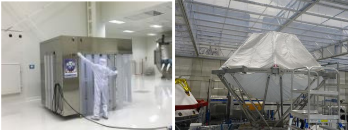
Figure 5-28: Portable tent examples used in cleanrooms during ALD (Analytical Laboratory Drawer) and ExoMars 2016 EDM (Entry Descent Module) activities
