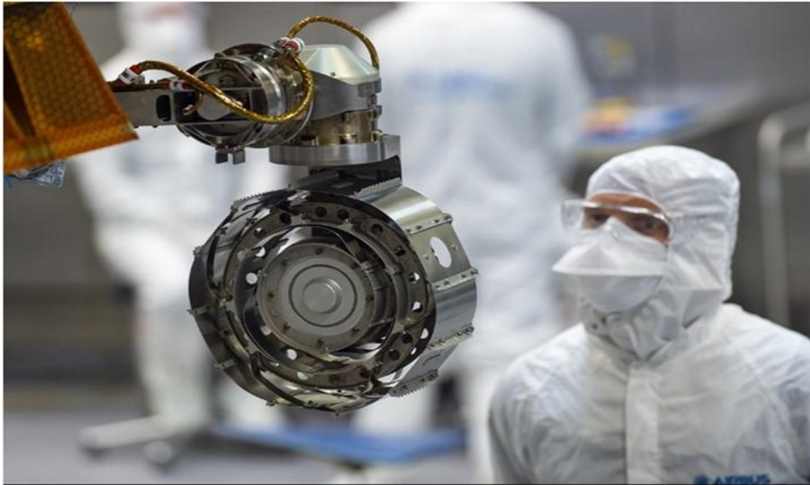
Figure 5-52: Detail of the bogies electro-mechanical actuator and complex geometry of wheels of the ExoMars Rosalind Franklin Rover. Credit: Airbus UK
