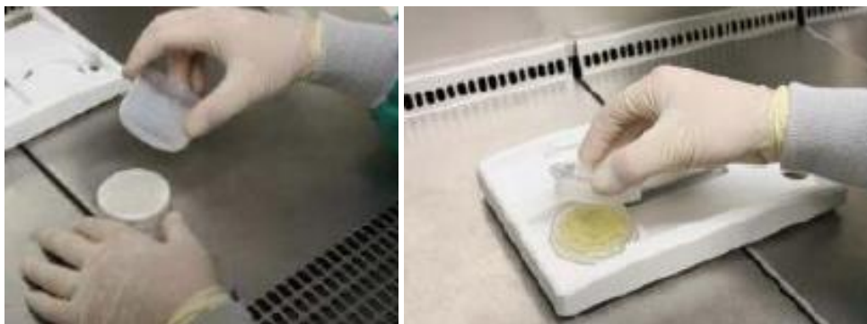
Figure 5-45: Funnel is removed from pump head and membrane (left); the membrane (0,45 µm) is transferred onto R2A or TSA nutrient agar cassette
